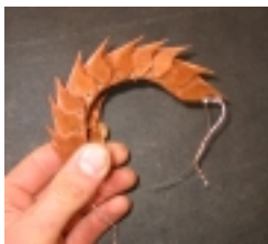
Figure 5.3: Copper leaf prototype. The leaf is actuated by a pull on the string.
